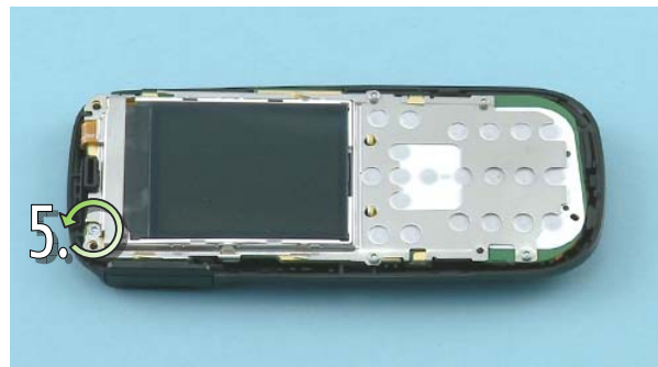
6) Tighten the remaining Torx+ 4 screw to the torque of 12 Ncm.
