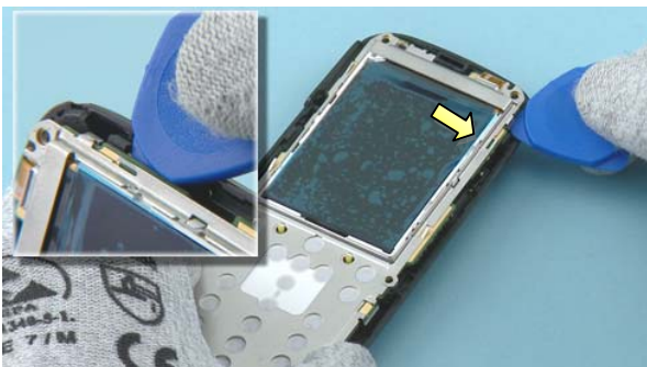
11) Separate the ENGINE MODULE from the D-COVER by releasing the first clip using the SRT-6.
