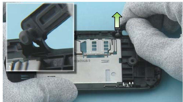
18) Remove EF II COVER by pulling it out gently in the direction shown.
