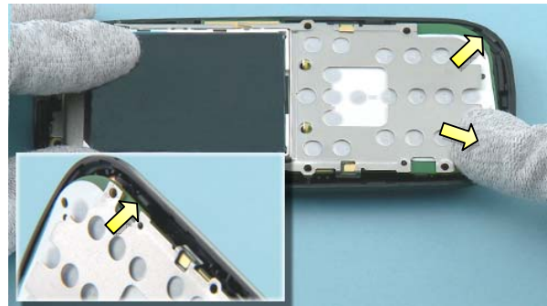
4) Then press gently on the lower ends of the ENGINE MODULE to lock with the two snaps on the D-COVER.
